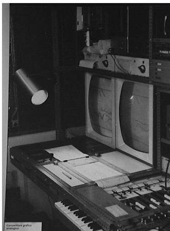
Figure 2. The Analog Graphic Converter developed by Fernando von Reichenbach at CLAEM during the late 60s.
